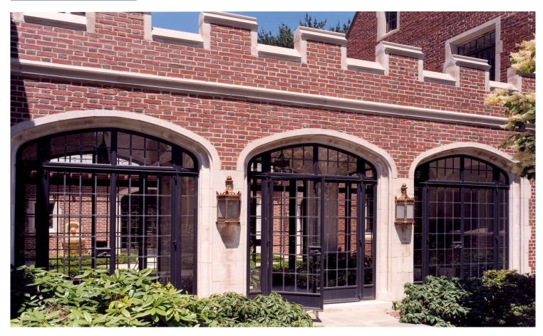
The Berkeley window and door system is an ideal solution for historic projects where minimum sightlines, maximum daylight, and fine detail are desired. Hot rolled profiles feature an external solid steel chamfer that replicates traditional putty glazing in combination with internal beading that offers security and access for re-glazing.
